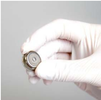
iButton humidity datalogger
